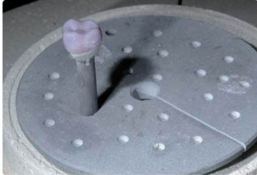
Place the glazed and stained restoration into the centre of the IPS e.max CAD Crystallization Tray
