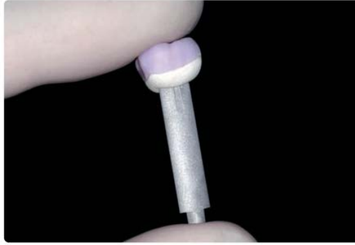
Press the selected IPS e.max CAD Crystallization Pin deeply into the IPS Object Fix Putty or Flow
