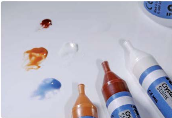
Extrude IPS e.max CAD Crystall./Shades and Stains from the syringe and mix thoroughly. If required, thin with IPS e.max CAD Crystall./Glaze Liquid
