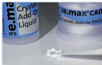
Mix IPS e.max CAD Crystall./Add-On with IPS e.max CAD Crystall./Add-On Liquid to an easy-to-contour consistency.
