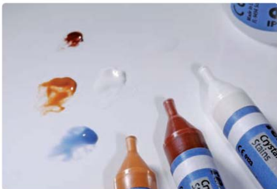
Extrude IPS e.max CAD Crystall./Shades and Stains from the syringe and mix thoroughly. If required, thin with IPS e.max CAD Crystall./Glaze Liquid
