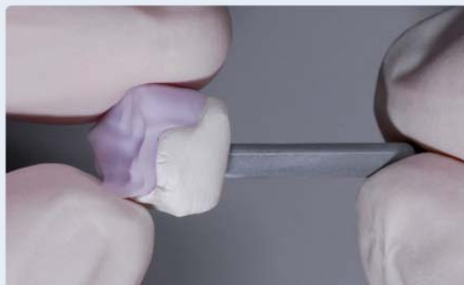
Press the suitable IPS e.max CAD Crystallization Pin into the Putty or Flow material
