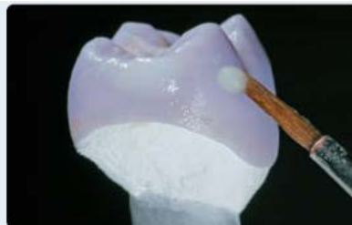
Application of the mixed Add-On on the blue restoration before crystallization
