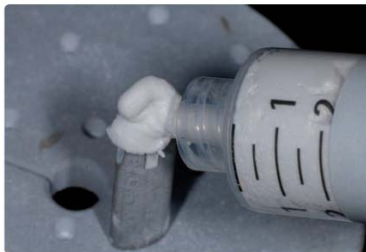
Apply IPS Object Fix Flow on the IPS e.max CAD Crystallization Pin.
