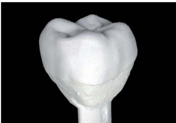
Allow the IPS e.max CAD Crystall./Glaze Spray to dry briefly until a whitish layer has formed. If required, spray the restoration again to achieve an even Glaze Spray layer on the IPS e.max CAD restoration.
