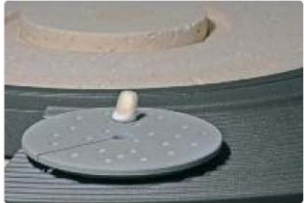
Remove the crystallization tray from the furnace once the crystallization program has been completed and allow the IPS e.max CAD restoration to cool to room temperature
