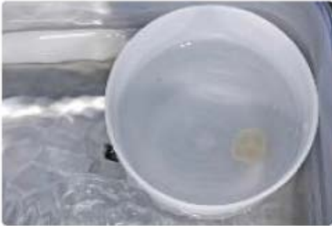
Remove residus with ultrasound in a water bath...
