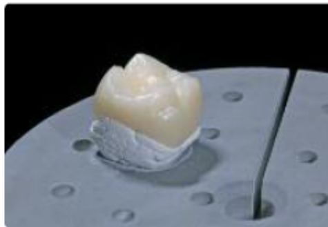
Remove the crystallization tray from the furnace once the crystallization program has been completed, and allow it to cool
