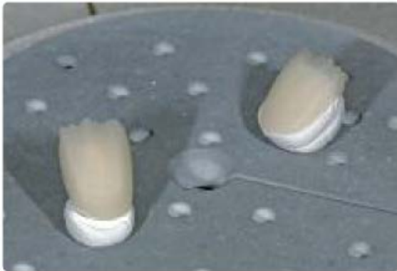
Remove the crystallization tray from the furnace once the crystallization program has been completed and allow it to cool to room temperature
