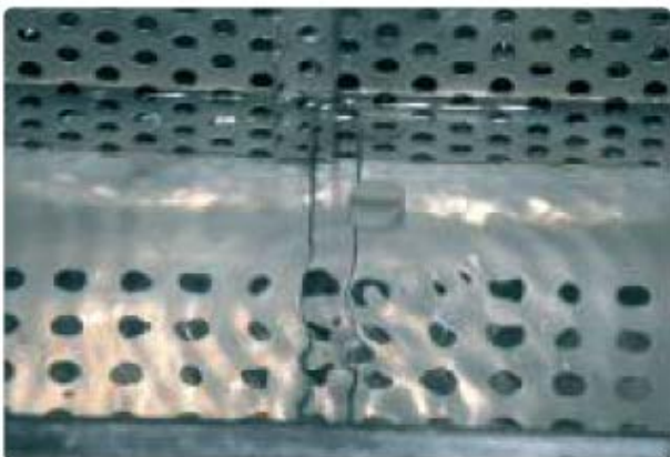
Remove any residue with ultrasound in a water bath and/or with steam
