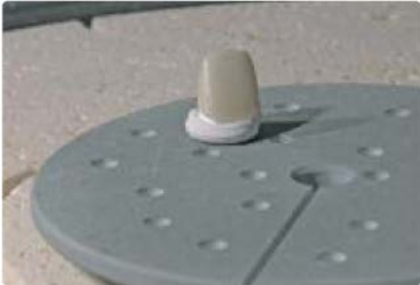
Remove the crystallization tray from the furnace once the crystallization program has been completed and allow the IPS e.max CAD restoration to cool to room temperature
