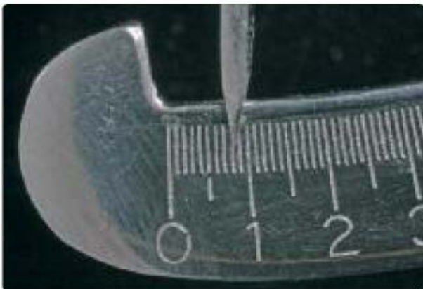
Make sure that the minimum thicknesses are maintained even after finishing
