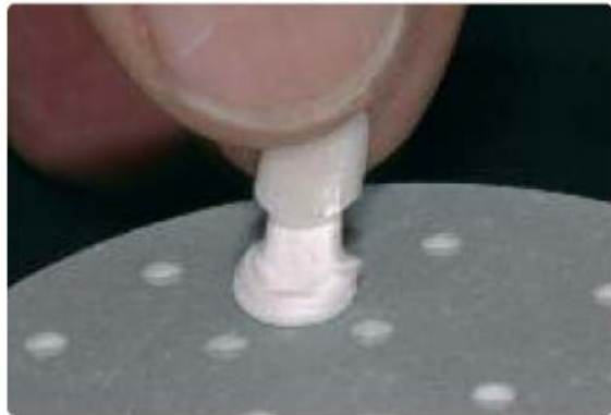
Remove the restoration from the hardened auxiliary firing paste
