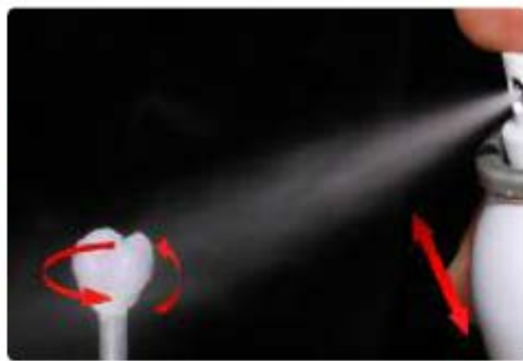
Spray the IPS e.max CAD Crystall/Glaze Spray directly on the unfired IPS e.max CAD Crystall/Shades and Stains. Spray the restoration from all sides while simultaneously rotating it.
