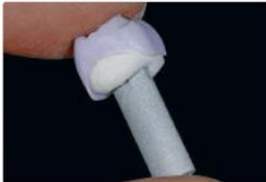
Press the selected IPS e.max CAD Crystallization Pin deeply into the IPS Object Fix Putty or Flow material
